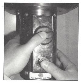
If for some reason your igniter fails to deliver a spark, your heater can be started by inserting a lit match through the pilot view hole while pushing the control knob in while in the PILOT position.
